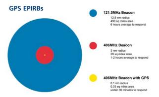
The GPS EPIRB and PLB have been designed to enhance further the lifesaving capabilities of conventional beacons. The standard Global Positioning System (GPS) uses an array of 27 satellites and provides continuous positional information with a typical accuracy of around 50m. A 406MHz EPIRB such as the Smartfind Plus or PLB such as the Fastfind Plus has a built in GPS, when the beacon is activated in an emergency, positional information is incorporated into the distress message which it transmits.
